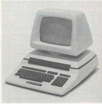
The Commodore 700 or B series is a software compatible range of professional computers starting with 128K of user memory (RAM). This series features an attached display and integral disk units.
